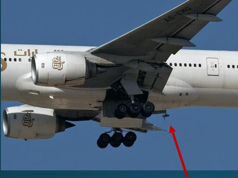
B777-200ER in flight with deployed RAT
